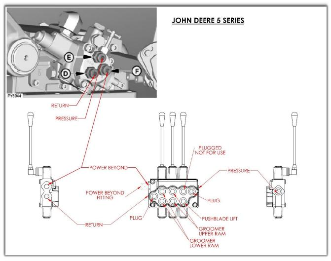
A-Fitting B-Fitting C-Fitting D-Fitting, Return Oil Line E-Fitting, Pressure Oil Line F-Fitting, Power Beyond
